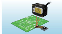
Example of an application that does not require the entire measurement range Low-profile connector assembly height measurement
