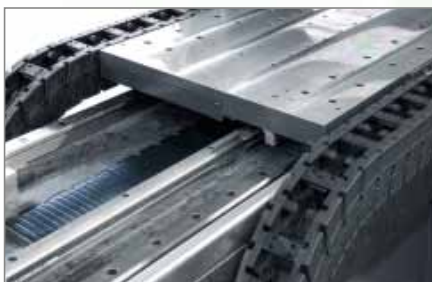
Iron core linear motor components in laser processing for precise, uniform movement of the substrate and laser.
