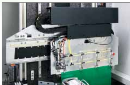
Iron core linear motor components in printed circuit board processing for high dynamic and precise positioning of tools and PCBs.
