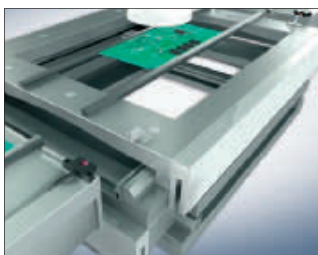
Easy to mount end position detection / limit sensors (contactless).
