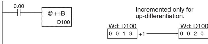
The up-differentiated variation is used in the following example, so the BCD content of D101 and D100 will be incremented by 1 only when CIO 0.00 has gone from OFF to ON.
