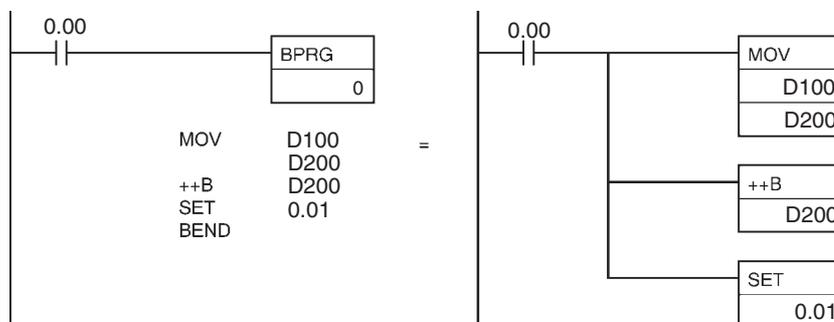
The two program sections shown below both execute MOV(021), ++B(594), and SET for the same execution condition (i.e., when CIO 0.00 turns ON).
