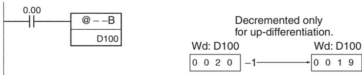
The up-differentiated variation is used in the following example, so the BCD content of D101 and D100 will be decremented by 1 only when CIO 0.00 has gone from OFF to ON.
