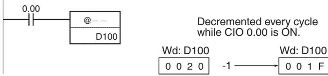
The up-differentiated variation is used in the following example, so the content of D101 and D100 will be decremented by 1 only when CIO 0.00 has gone from OFF to ON.
