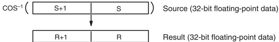
The result is output to words R+1 and R as an angle (in radians) within the range of 0 to  $\pi$ .
