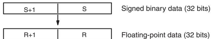
Signed binary data within the range of  $-2,147,483,648$  to  $2,147,483,647$  can be specified for S+1 and S. The floating point value has 24 significant binary digits (bits). The result will not be exact if a number greater than  $16,777,215$  (the maximum value that can be expressed in 24-bits) is converted by FLTL(453).
