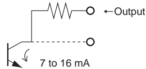
(2) Open collector output with 1.6-kΩ limit resistance
