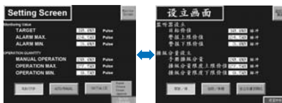
Example: The label switch function can be used to switch between English and Simplified Chinese.
