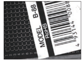
Automatically choosing the most appropriate filter to prevent halation and generating images most appropriate for inspections
